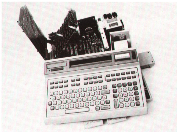
Fig. 1. 9825A Calculator is fully operational when opened for servicing. Printed circuit boards are hinged to provide access to both sides. Plug-in ROMs at front and side were pulled halfway out for this photo.
